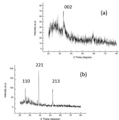
**Fig. 3** the XRD of the (a) ZnO nanoparticle (b)  $(\text{CH}_3\text{NH}_3)\text{PbI}_3$  perovskite thin film on glass substrate.
