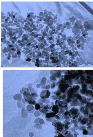
Fig.4 Transmission Electron Microscopy (TEM) of ZnO nanoparticles.
