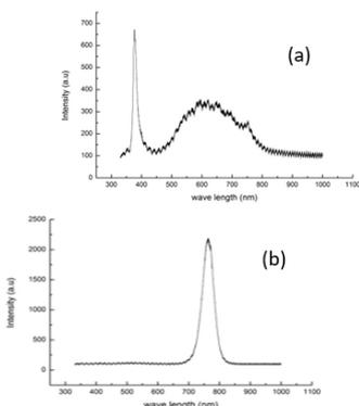
**Fig. 2** The photoluminescence (PL) spectrum of (a) ZnO nanoparticles. (b)  $(\text{CH}_3\text{NH}_3)\text{PbI}_3$  perovskite film on glass substrate.
