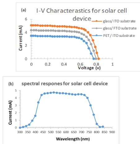
Fig. 6 (a) the current - voltage (I-V) curves of the perovskite solar cells. (b) The spectral response of solar cell device.
