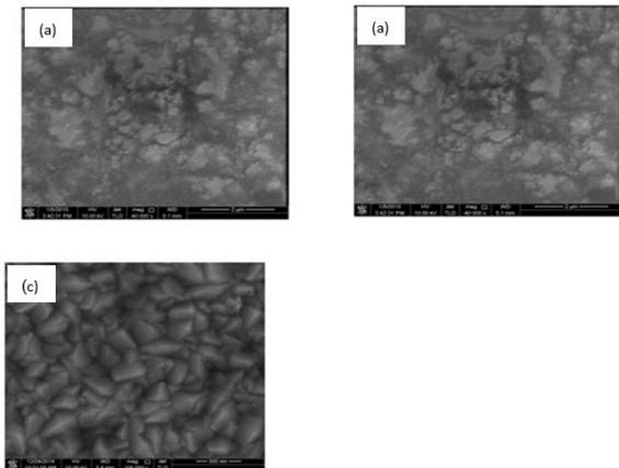
Fig. 5 the (FESEM) surface morphology for the (a) ITO/ZnO (NP). ((b) ITO/ZnO (NP)/PbI<sub>2</sub>, (c) ITO/ZnO (NP) / (CH<sub>3</sub>NH<sub>3</sub>)PbI<sub>3</sub> perovskite.
