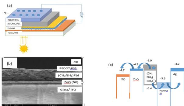
**Fig. 1** Device architecture of glass/ITO/ZnO (NP)/Perovskite/PEDOT:PSS/Ag. Solar cell (a) schematic of the device structure. (b) FESEM cross-section image of the device. (c) Energy level diagram.
