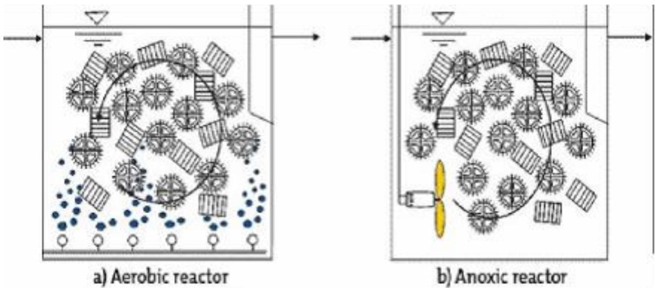
Figure 7 The typical reactors of MBBRs with submerged and suspended packing material [3, 6]
