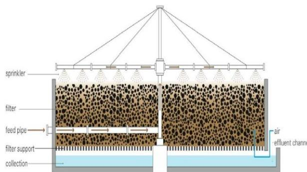
Figure 2 Typical trickling filter [6]
