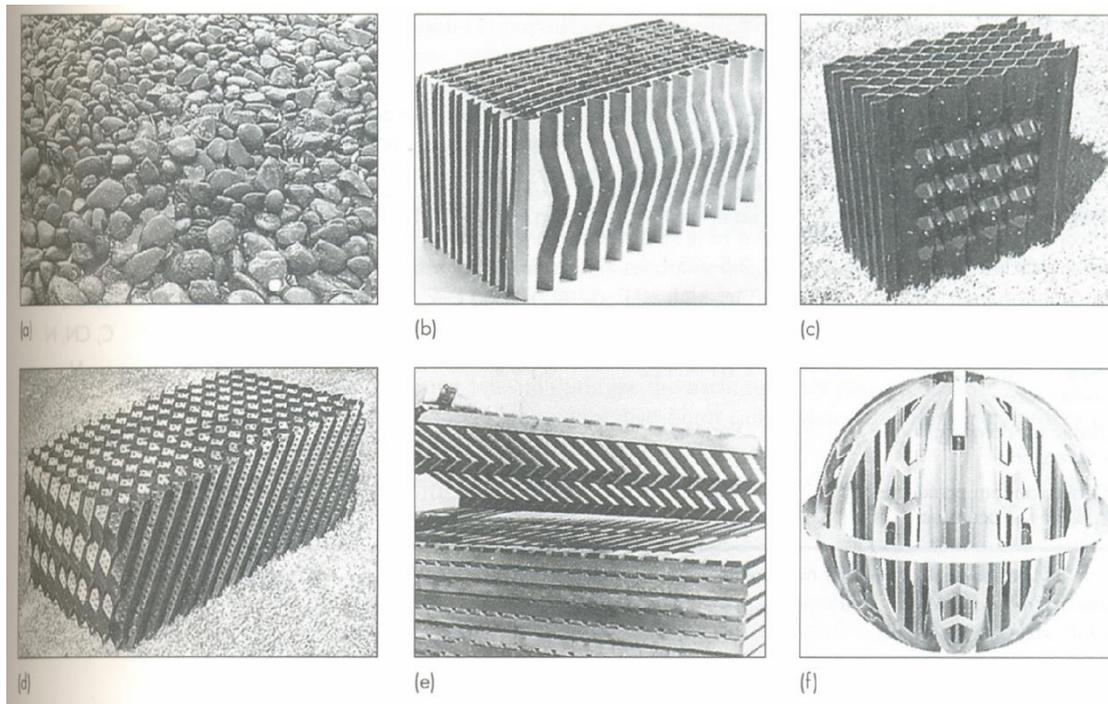
Figure 3 Typical packing material for trickling filters: (a) rock, (b) and (c) plastic vertical-flow, (d) plastic cross-flow, (e) redwood horizontal, and (f) random pack. [3]
