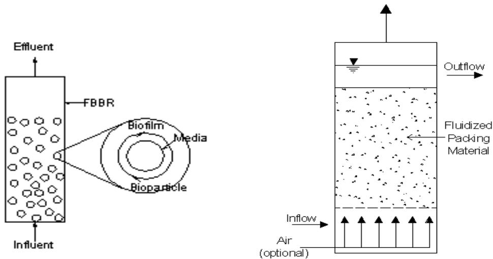
Figure 6 schematic fluidized bed reactors a) anaerobic FBR b) aerobic FBR [3, 35]
