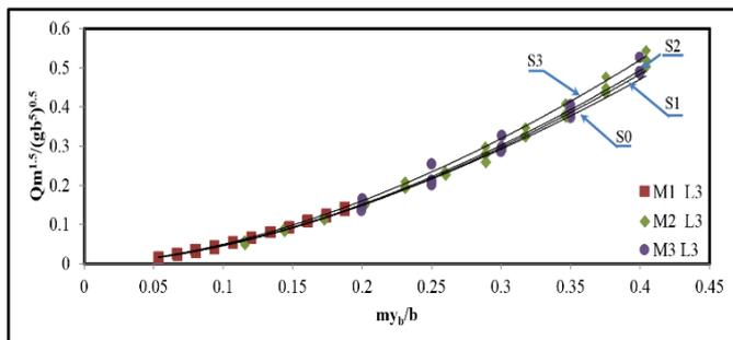
Figure 6. Variation of  $(Qm^{1.5}/\sqrt{gb^5})$  with  $(my_b/b)$  for different bed slopes of roughness pattern (L3)
