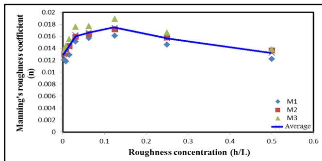
Figure 5. Variation of Manning’s roughness coefficient with roughness concentration (h/L)
