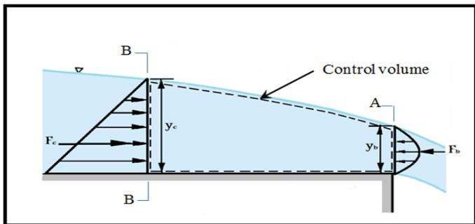
Figure 1. Control volume for theoretical analysis
