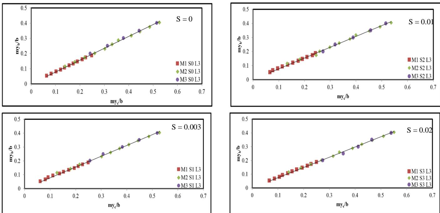
Figure 7. Variation of  $(my_b/b)$  with  $(my_c/b)$  for different bed slopes and roughness pattern (L3)
