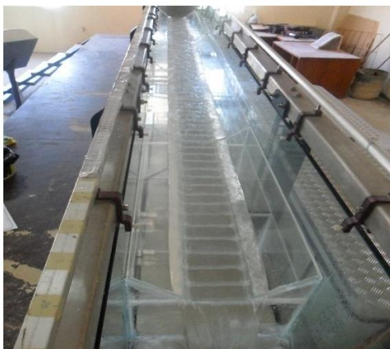
Figure 4. Rough bed model during a test run
