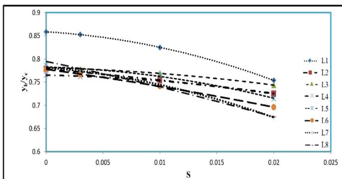
Figure 8. Variation of  $(y_b/y_c)$  with bed slopes (S) for different roughness patterns.
