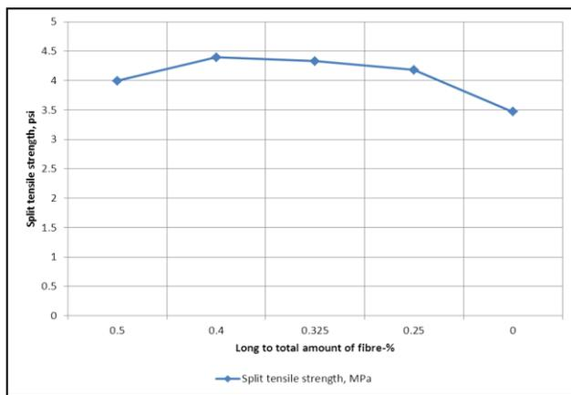
FIGURE 4. INFLUENCE OF LONG TO TOTAL AMOUNT OF FIBRE RATIO ON THE SPLIT TENSILE STRENGTH AT 28 DAYS
