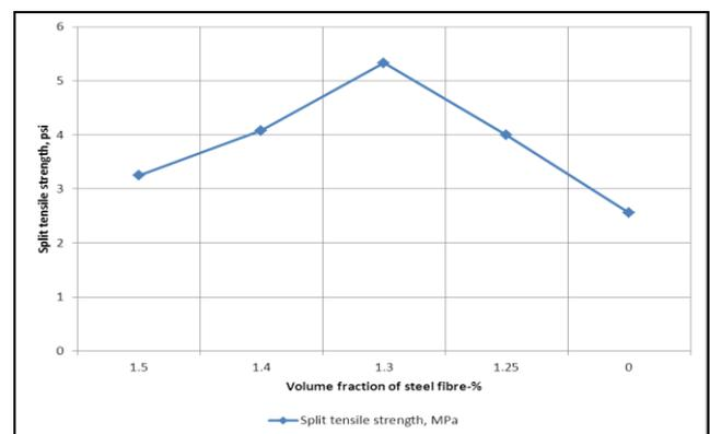
FIGURE 2. INFLUENCE OF VOLUME FRACTION OF COMBINED FIBRES ON THE SPLIT TENSILE STRENGTH AT 28 DAYS
