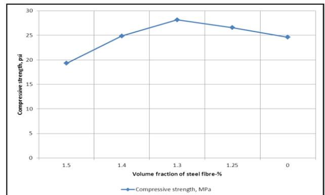
FIGURE 1. INFLUENCE OF VOLUME FRACTION OF COMBINED FIBRES ON THE COMPRESSIVE STRENGTH AT 28 DAYS
