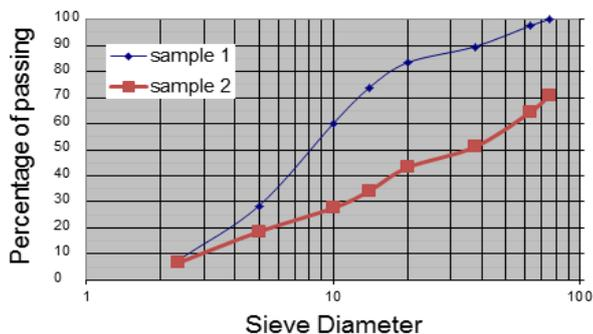
Figure4. Seive Analysis for two samples of soil
