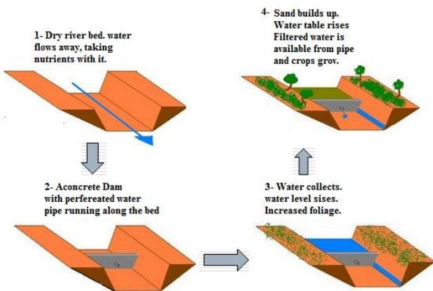
Figure2. The Mechanism of Sand Storage Dam
