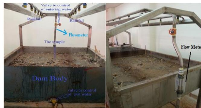
Figure3. The model of Sand Storage Dam
