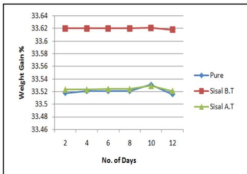
Figure 5. weight gain% of composites (polyester- sisal fiber as a function of time squared for salt solution before &after treatment
