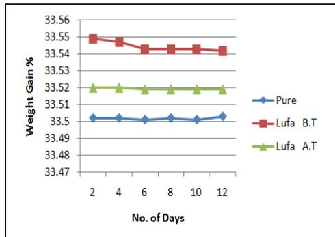
Figure 6. weight gain% of composites (polyester- lufa fiber as a function of time squared for salt solution before &after treatment.
