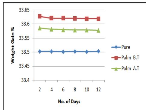
Figure 7. weight gain% of composites (polyester- palm leaf as a function of time squared for salt solution before &after treatment.
