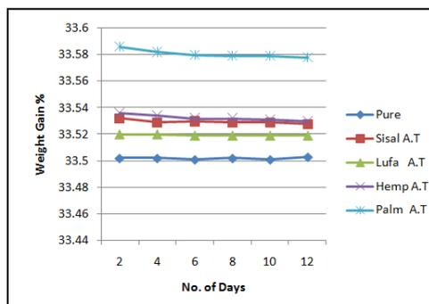
Figure 4. weight gain% of composites after treatment as a function of time squared for salt solution.
