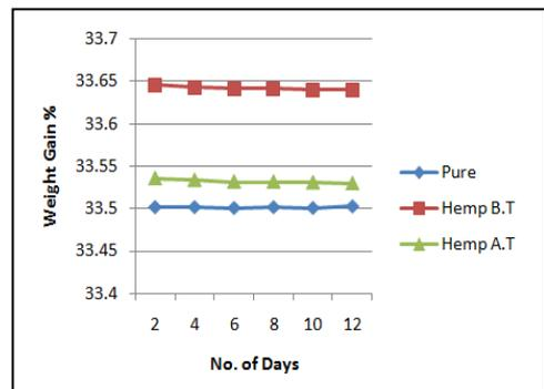
Figure 8. weight gain% of composites (polyester- Hemp fiber as a function of time squared for salt solution before &after treatment.
