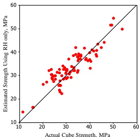
Figure (8) Predicted versus measured compressive strength by equation (5)
