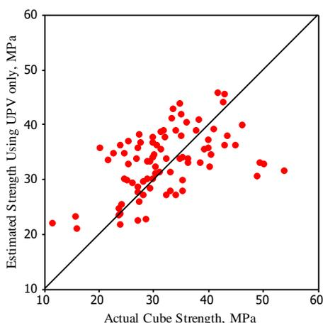
Figure (9) Predicted versus measured compressive strength by equation (6)
