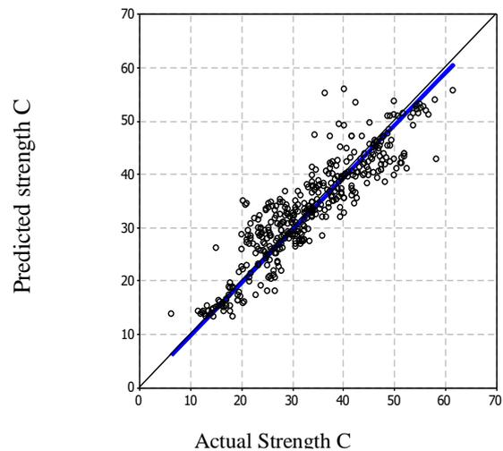
Figure (5) Predicted versus actual compressive strength by equation (1)
