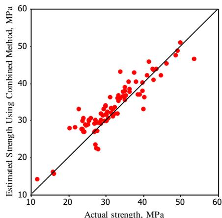
Figure (10) Predicted versus measured compressive strength by equation (7)
