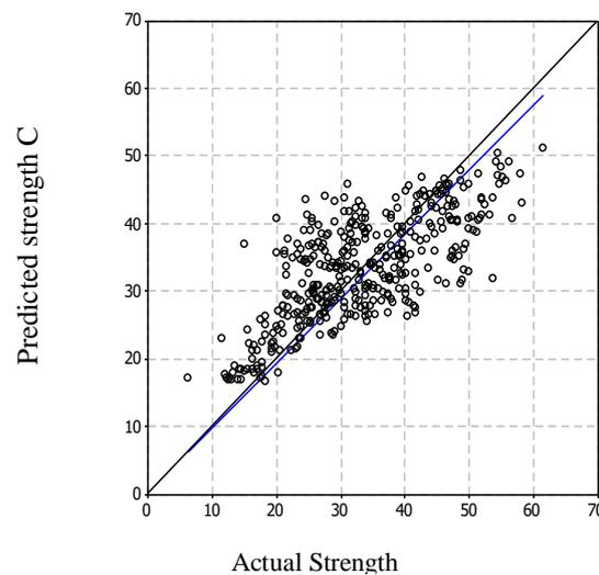
Figure (6) Predicted versus actual compressive strength by equation (2)
