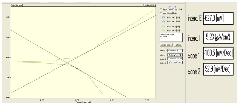
Figure 5. Polarization curves for (AA6061) Al /9% nano SiC composite in 3.5% NaCl.
