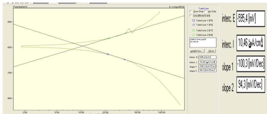
Figure 3. Polarization curves for (AA6061) Al /3% nano SiC composite in 3.5% NaCl.
