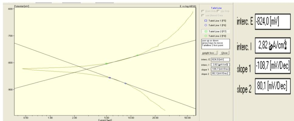
Figure 6. Polarization curves for (AA6061) Al /12% nano SiC composite in 3.5% NaCl.
