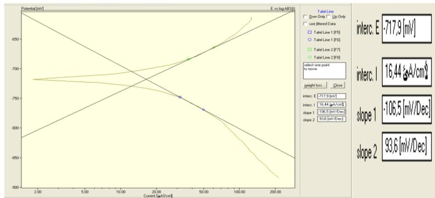
Figure 2. Polarization curves for (AA6061) aluminum alloy in 3.5% NaCl.
