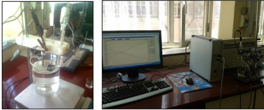
Figure 1. Experimental set up for electrochemical measurement.
