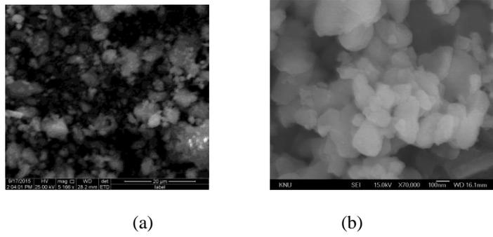
Figure 7 . SEM micrographs of (a) Al 6061 matrix powder and (b) SiC particles.
