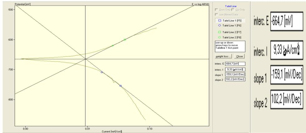
Figure 4. Polarization curves for (AA6061) Al /6% nano SiC composite in 3.5% NaCl.
