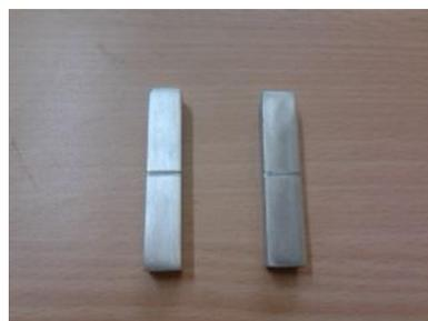
Figure 3. Samples for charpy impact test
