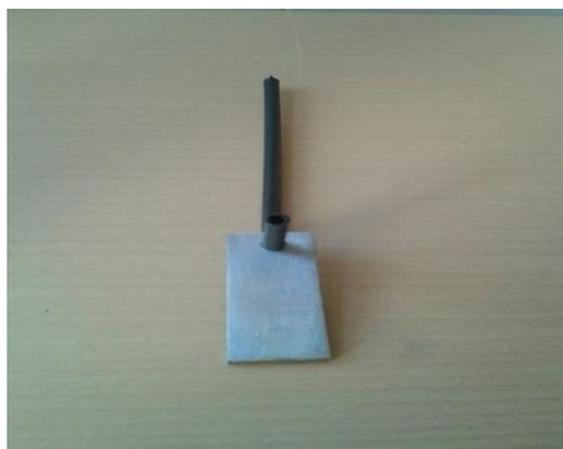
Figure 4. Sample for weigh loss tests
