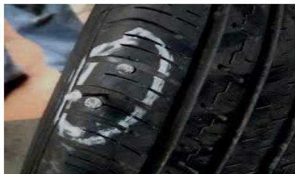
Figure 3. It can be seen nail Penetrated the tire layers
