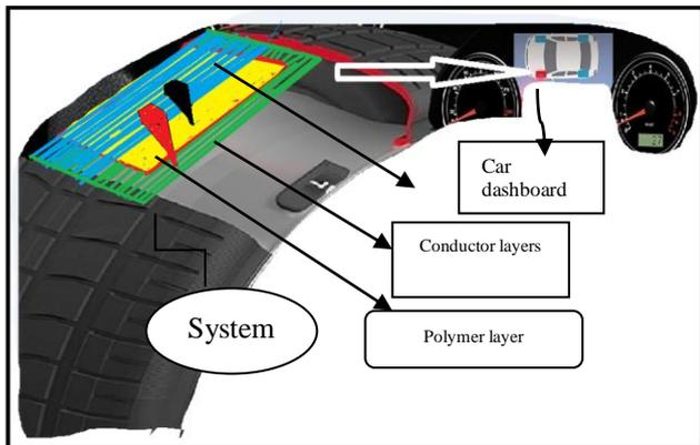
Figure 1. Visual Structure shows the Penetrated tire
