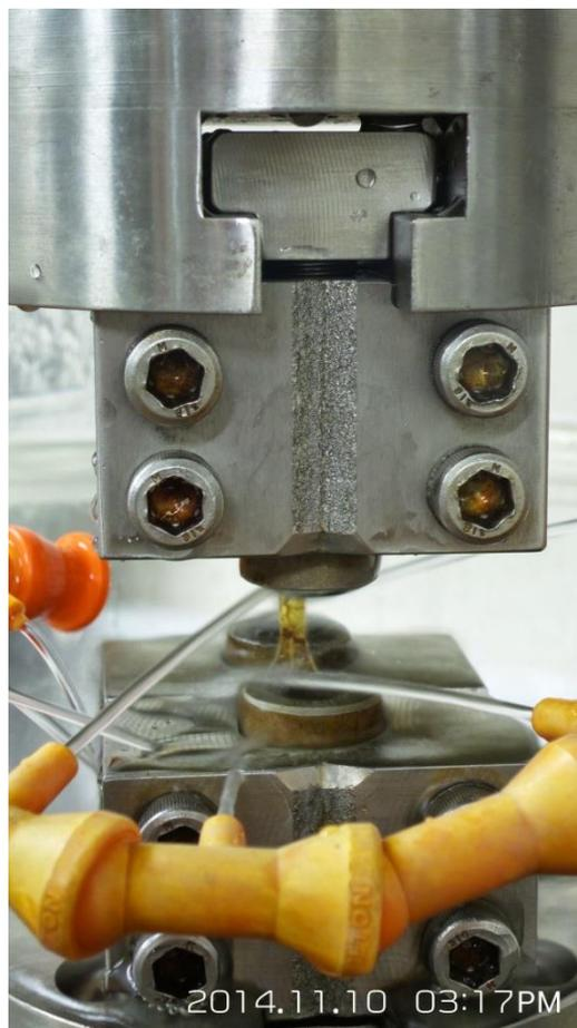
Figure 4 A 5coir/95epoxy green composite sample during the tension test under a flow of PBS at 37 °C.
