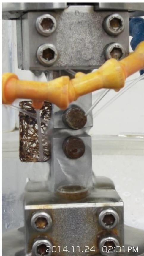
Figure 5 A 10coir/90PMMA green composite sample during the compact tension test under a flow of PBS at 37 °C.
