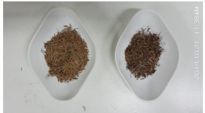
Figure 2 Coir natural fiber: before (left) and after (right) alkali treatment.
