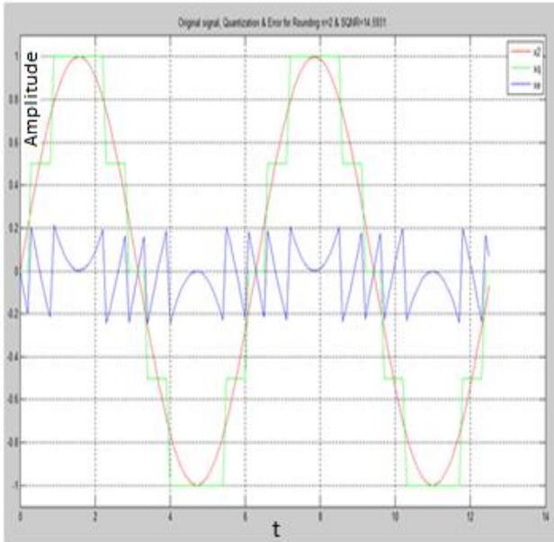
Figure 1. Original analog sine signal, Quantization and error using Rounding method for number of bits (n=2)
