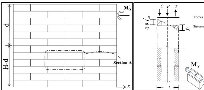
Figure 5 Typical masonry wall under the action of  $M'_y$
