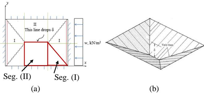
Figure 3 (a) wall divided into triangular and rectangular segments, (b) three-dimensional sketch of displaced wall.
