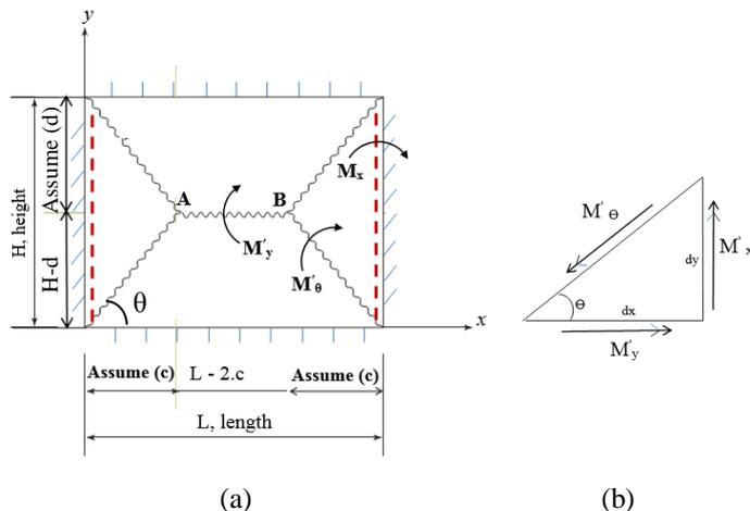
Figure 2 (a) assumed yield line pattern, (b) transformation of the plastic moment along inclined yield line into two moment components along x, and y axes.
