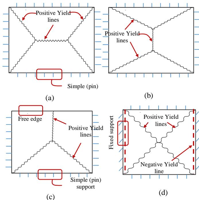
Figure 1 Yield line patterns in masonry walls; (a), and (b) rectangular with simple-support B.C; (c) rectangular with one free edge, (d) square with two fixed B.C
