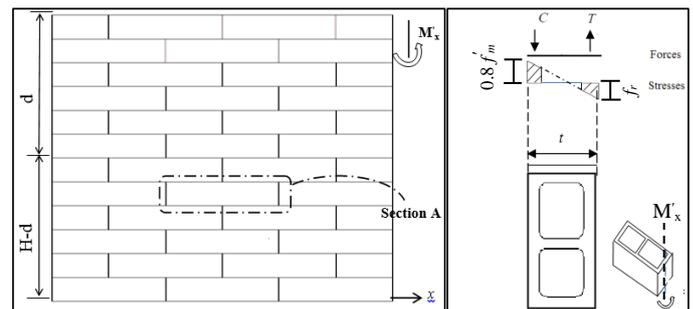
Figure 4 Typical Masonry wall under the action of  $M_x$  or  $M'_x$
