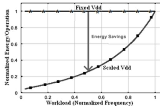
Fig. 3. Normalized energy vs. normalized frequency
