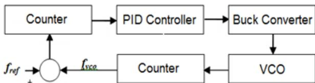
Fig. 4. The Block diagram of the DVS control loop
