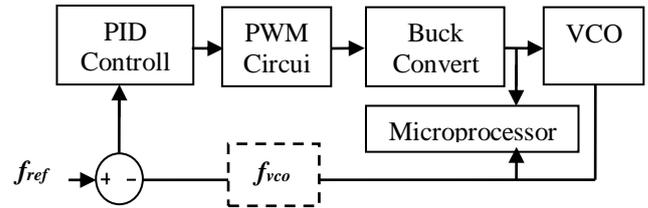
Fig. 2. Schematics of the simplified DVS unit
