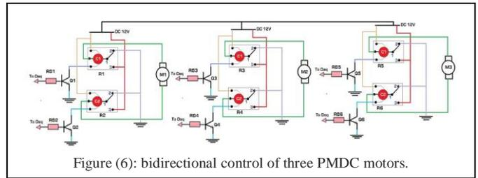
Figure (6): bidirectional control of three PMDC motors.
