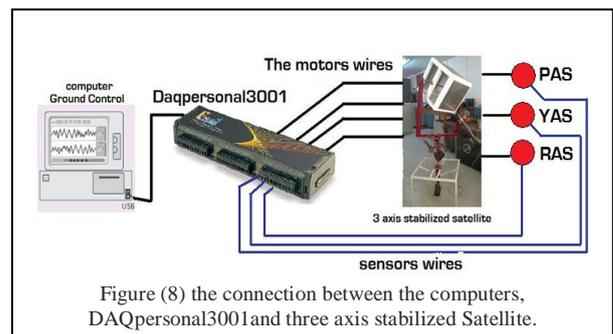
Figure (8) the connection between the computers, DAQpersonal3001 and three axis stabilized Satellite.
