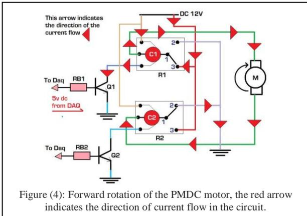
Figure (4): Forward rotation of the PMDC motor, the red arrow indicates the direction of current flow in the circuit.
