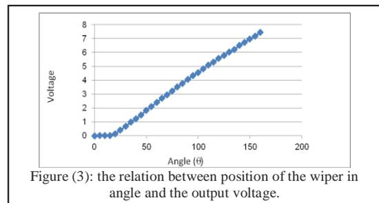
Figure (3): the relation between position of the wiper in angle and the output voltage.
