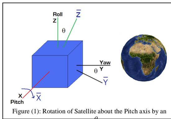
Figure (1): Rotation of Satellite about the Pitch axis by an  $\theta$
