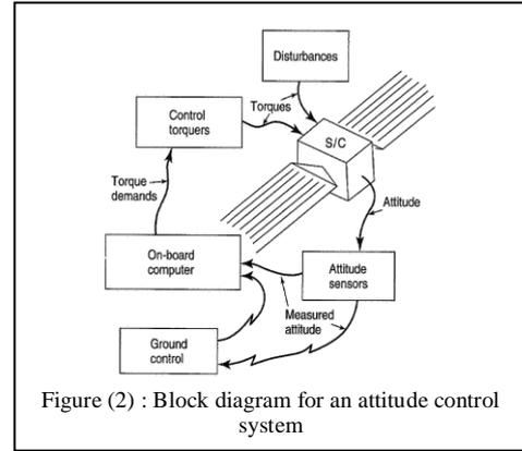
Figure (2) : Block diagram for an attitude control system
