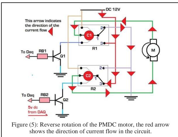
Figure (5): Reverse rotation of the PMDC motor, the red arrow shows the direction of current flow in the circuit.
