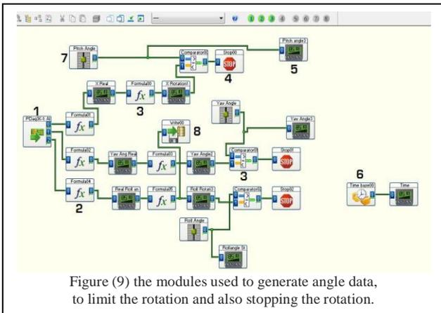
Figure (9) the modules used to generate angle data, to limit the rotation and also stopping the rotation.
