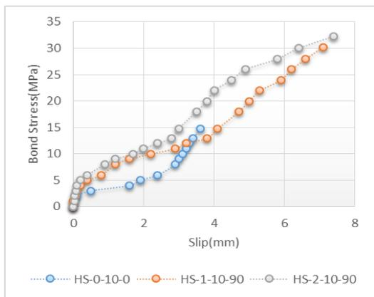
FIG.7 EFFECT OF FIBER CONTENT  $V_f$  ON BOND SLIP RESPONSE FOR GROUP C WITH AN ASPECT RATIO (L/D) =90
