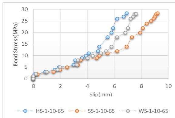
FIG. 10 EFFECTS OF FIBER SHAPES ON BOND SLIP RESPONSE FOR CONCRETE.
