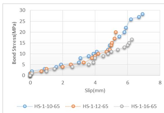
FIG 11 EFFECT OF BAR DIAMETER ON BOND SLIP RESPONSE
