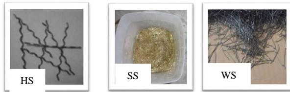
PLATE 2 TYPES OF STEEL FIBERS USED IN SFRC
