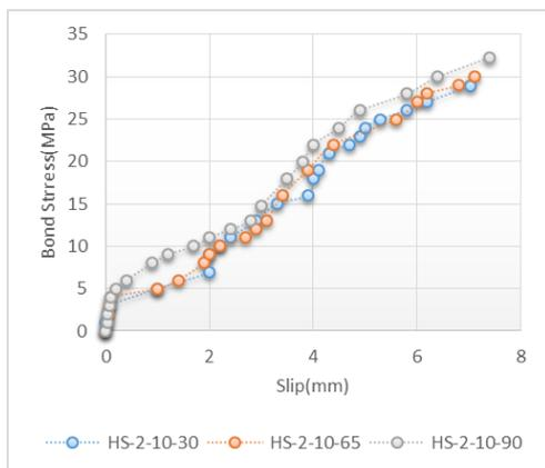
FIG. 9 EFFECT OF AN ASPECT RATIO (L/D) ON BOND SLIP RESPONSE FOR CONCRETE WITH FIBER CONTENT  $V_f = 2\%$
