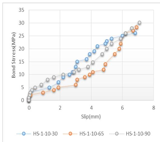
FIG. 8 EFFECT OF AN ASPECT RATIO(L/D) ON BOND SLIP RESPONSE FOR CONCRETE WITH FIBER CONTENT  $V_f = 1\%$
