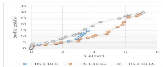
FIG.6 EFFECT OF FIBER CONTENT  $V_f$  ON BOND SLIP RESPONSE FOR GROUP B WITH AN ASPECT RATIO ( $L/D$ ) =65
