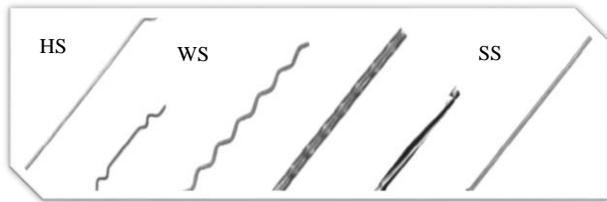
FIGURE 1 DIFFERENT TYPES OF STEEL FIBERS
