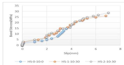
FIG. 5 EFFECT OF FIBER CONTENT  $V_f$  ON BOND SLIP RESPONSE FOR GROUP A WITH AN ASPECT RATIO ( $L/D$ ) =30
