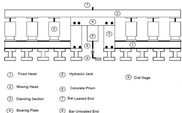
FIG. 3 TESTING FRAME DETAILS MACHINE.
