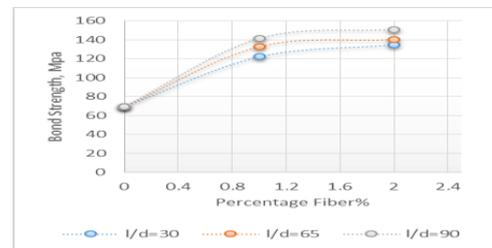
FIG. 4 EFFECT OF FIBER CONTENT ON BOND STRENGTH.
