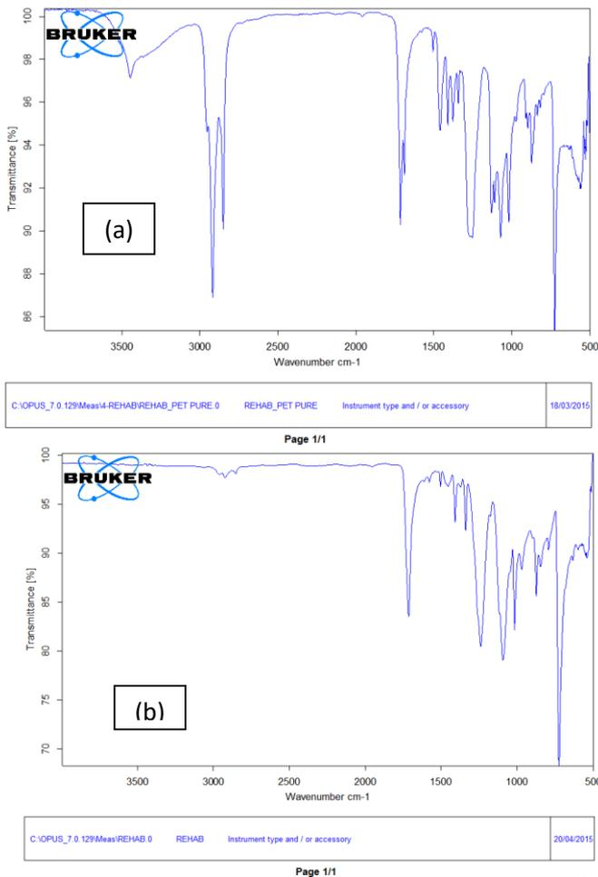
Figure 5. The FTIR spectrum of the glycolysed (a), & pure Bottle (b).
