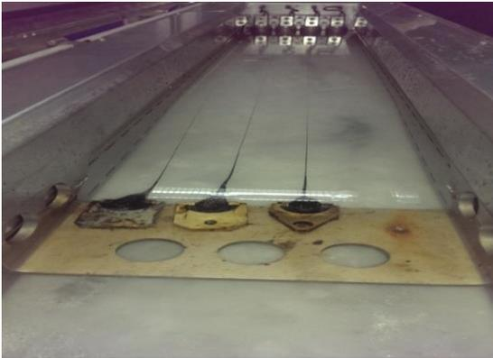
Figure 3. Ductility testing machine.
