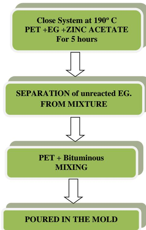
Figure 2. Flow diagram of experimental work.
