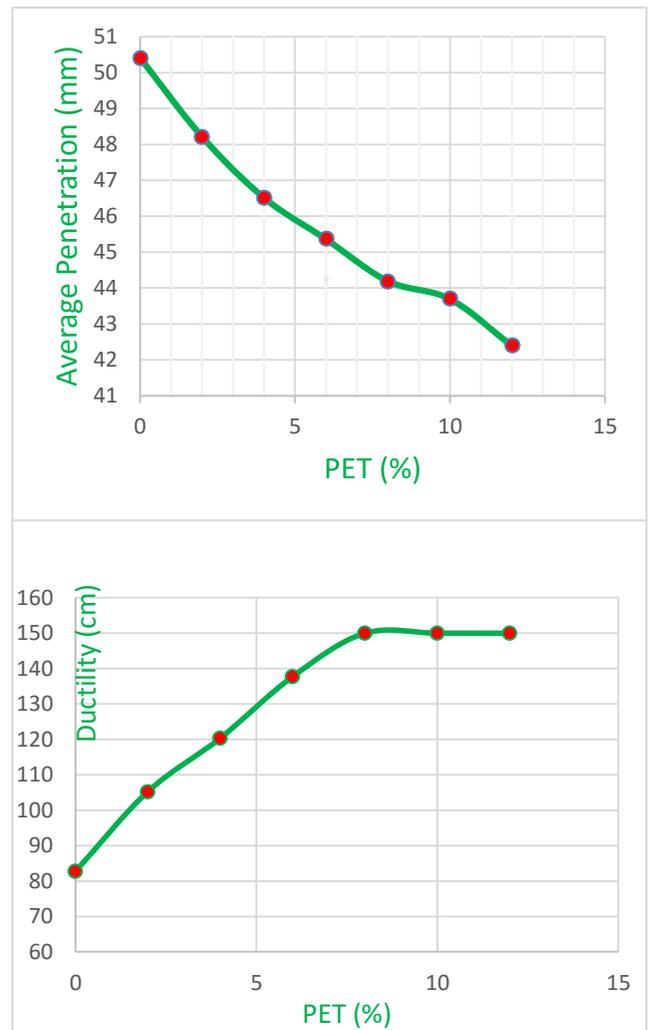
Figure 4. Ductility and Penetration Vs PET additive
