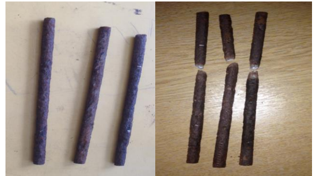
Figure 2. Three steel bar specimen before and after tension test.
