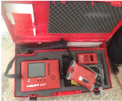
Figure 3. Ferro scan device and Reinforcement details scanning.
