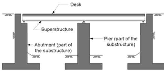
Figure 2: The primary component for a bridge
